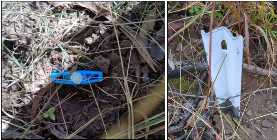
Photo 2: Survey pegs at start (0 m) and mid-point (50 m) of permanent monitoring sites
